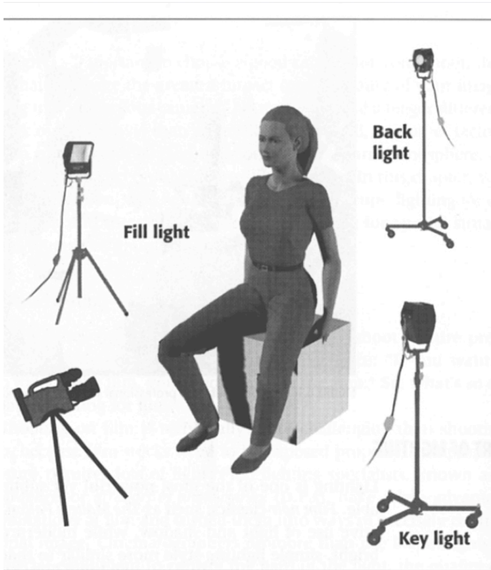
FIGURE 6.2 A diagram of a typical three-point lighting setup, including camera placements and subject.
